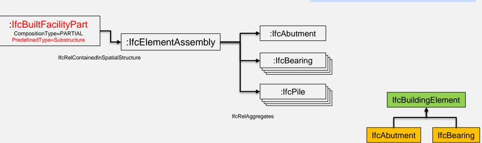
New Elements IfcAbutment, IfcBearing?
